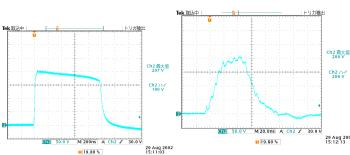
Input voltage: 2 kV Pulse width: 1000 ns Load: 50 ohm V: 50 V/div Input voltage: 2 kV Pulse width: 50 ns Load: 50 ohm V: 50 V/div H: 10 ns/div
