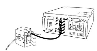
\* With 1kV or higher input, the unit may vibrate and generate sounds due to that but this is a normal behavior of this unit.
