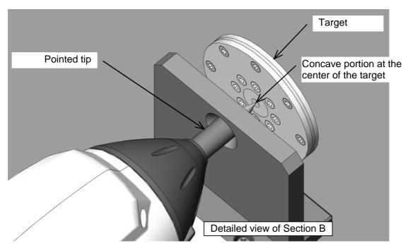
\* The figure shows the GT-30R(A) discharge gun. The setup is the same as with the TC-815R/S discharge gun.
