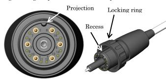
High voltage output connector of the electrostatic discharge simulator
