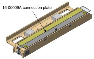
The ground (GND) plate of this unit is connected to the ground plate of the coupling clamp 15-00009A.
