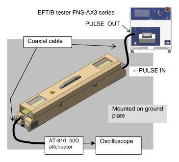
From PULSE OUT terminal of the tester, output a pulse with 2 kV setting value, and evaluate the waveform applied to the clamp calibration unit. Waveform evaluation: One pulse
