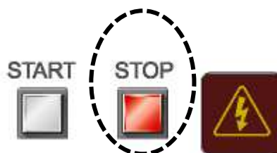
※Control Panel of the Impulse Noise Simulator
