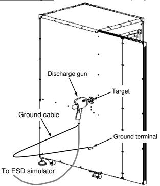
Set the discharge gun with a non-metal type gun holder (like Noiseken's 03-00061B) as the point of the discharge tip contacts perpendicularly to the center conductor of the Unit. Connect the ground cable of the discharge gun to the ground terminal of the Faraday cage with drawing the cable backward so that the cable can make two sides of an isosceles triangle.
