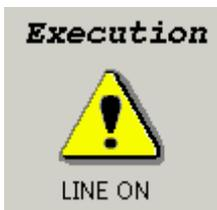
During testing, the Execution sign appears on the upper light of the screen and blinks to indicate that the test is in progress.
