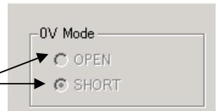
Select [SHORT]: MG22 is ON (MG21 is OFF) and outputs L1-L2 short 0 V.
