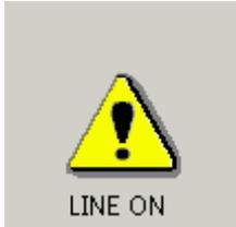
When <LINE> button pressed, this sign turns on (alight) on the upper right of the screen to indicate that the LINE is on.
