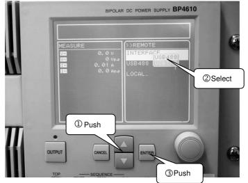
Install the driver software for the built-in amplifier(BP4610).
