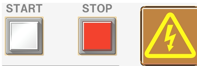
Figure 11-9 Operation Panel START and STOP Controls
