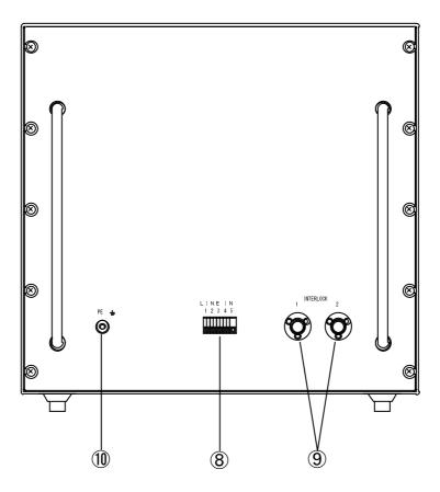
**®DC LINE IN TERMINAL [LINE IN]:** Inputs power for EUT.
