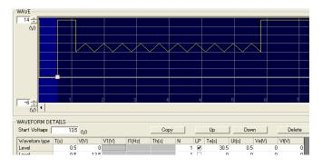
Easily and reliably creates a loop waveform using the sweep function detailed at left for a long test duration requiring varying T (times) and V (voltages).
