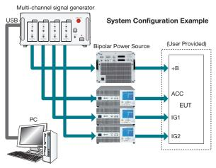
The system is primarily comprised of the following three elements: multi-channel signal generator, bipolar power source(s), and arbitrary waveform creation software.
