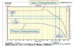
There is variation in 10kHz - 20k Hz range Gain variation of 2.5 dB is evident up to 100 kHz and variation of 3.5 dB up to 200 kHz.
