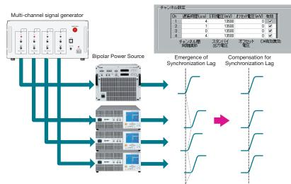
In multichannel tests it is important to ensure each individual channel is precisely synchronized. This system guarantees a synchronization delay of  $1\mu$ s or less by compensating for output timing differences from the power amplifiers being connected, whereas other systems are not equipped with similar capability, which often leads to a erroneous test.
