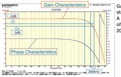
Gain characteristics stable to 100 kHz A slight deviation of 1 - 2dB up to 200kHz only
