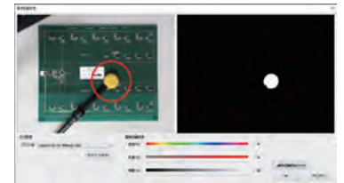
Image recognition (probe tip yellow color recognition)
