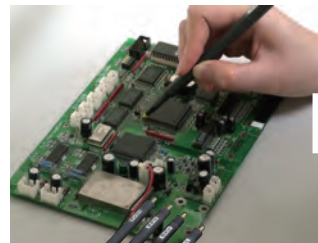
- Small precision probes - Small components and PCB EM field measurement
